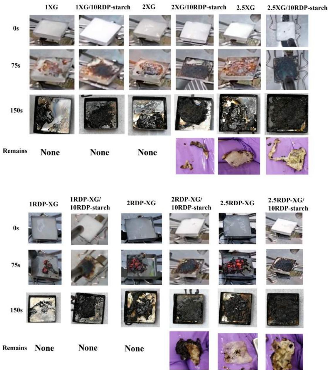
Fig. 5. Hydrogels at 0s, 75s, and 150s of flammability assessments and the recovered sheepskin remains.
