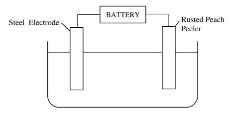
As current is applied to the cell, bubbles of oxygen gas form at the steel electrode, while the rust on the peach peeler is converted into a loose layer of a dark solid that Michael identifies as iron metal. By weighing the cell before and after the electrolysis is complete, Michael finds that 6.82 g of oxygen were evolved (recall that oxygen has an equivalent weight of 8).
