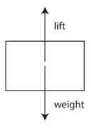
As the helicopter is hovering there is no horizontal thrust or air resistance.
