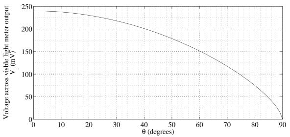
Angle between axes of two polarising filters
