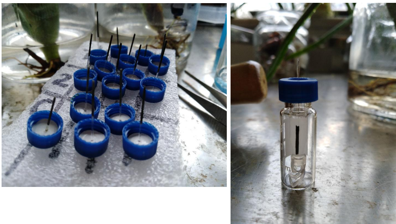
Figure 6 The appearance and assembly of C18@GO@PDDA SPME Fibers
