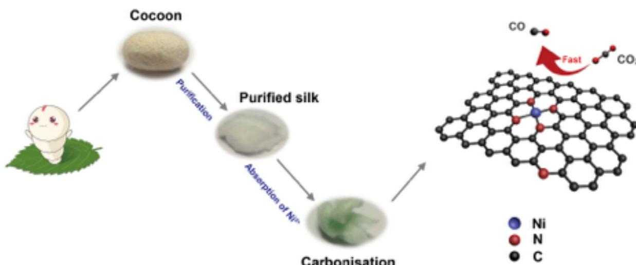
**Figure 1.** Scheme of experimental procedure and demonstration of electrochemical CO<sub>2</sub>RR reaction mechanism.
