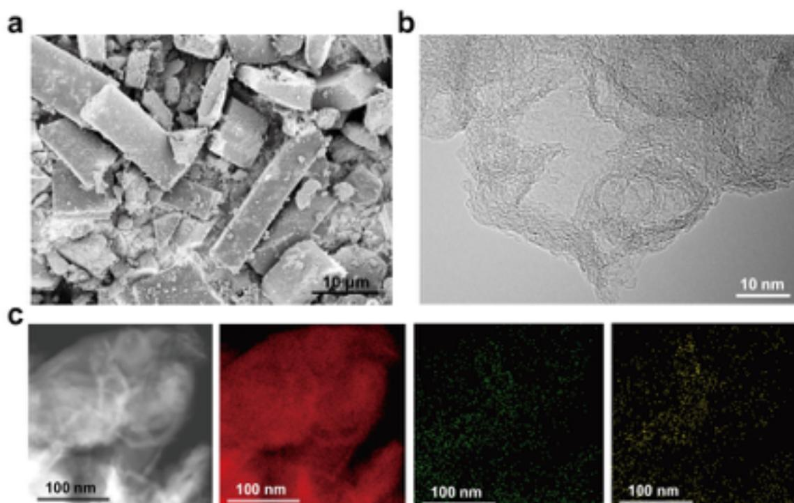
**Figure 2.** Structural Characterisation. (a) Scanning Electron Microscopy (SEM) of Carbonised  $\text{Ni}(\text{NO}_3)_2$  (DMF) Dipped Silk (Ni/N-C). (b) Transmission Electron Microscopy (TEM) of Ni/N-C. (c) Energy Dispersive Spectroscopy (EDS) elemental mapping of Ni/N-C. The red, green and yellow colours were denoted for C, N and Ni, respectively.
