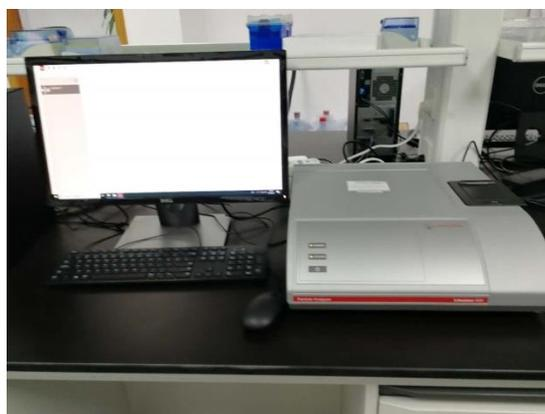
Figure 2.2. Nano Particle Size/Zeta Potential Analyzer in lab.
