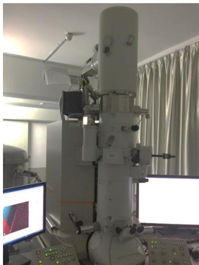
Figure 2.4. JEM-2100 Plus Field Emission Electron Microscope in University Testing Center.
