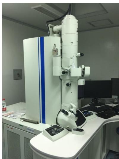
Figure 2.3. JEM-1400 Plus Electron Microscope in University Testing Center.
