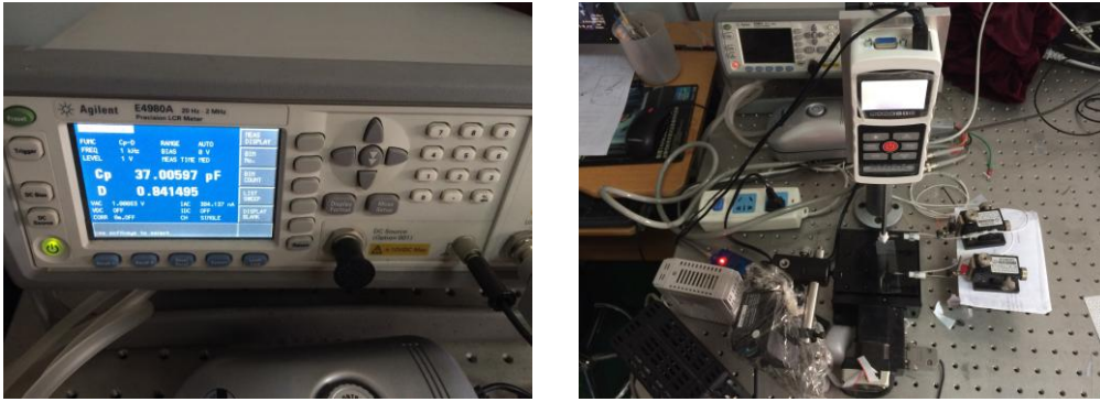
Figure 6.1 LCR type E4980A table (left) and test device group (right)
