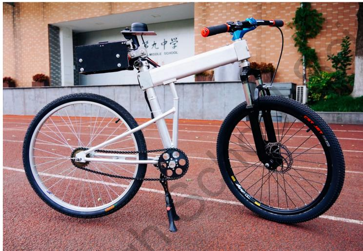
Figure 7: The autonomous self-balance electric bicycle.
