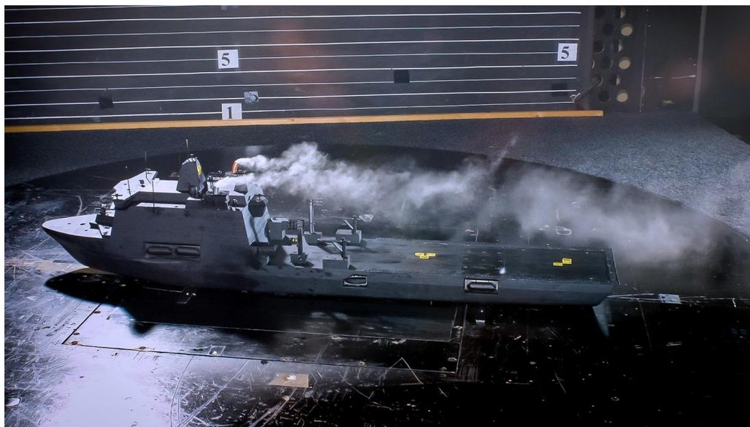
Figure 2: Wind tunnel concept. A picture that illustrates a wind tunnel that tests the stream line design and many physical datas of a ship.<sup>[11]</sup>
